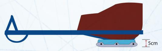
For a double amputee, the minimum length of the frame must be 80 cm and accommodate the front skid
