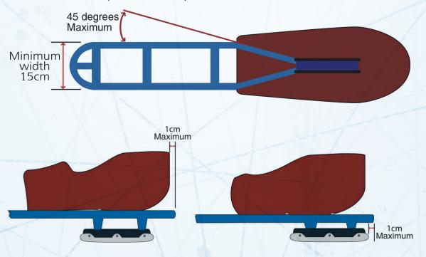
The front of the sled shall have a continuous curve with a maximum radius one half (1/2) of the inside width of the frame at its widest point forward of the seat. The following materials may be used in constructing this piece: Steel; Aluminum; Titanium; Magnesium, Polyurethane.
