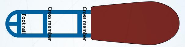
The height of the main frame measured from the ice to the bottom of the frame shall be a minimum 8.5 cm and maximum of 9.5 cm.
